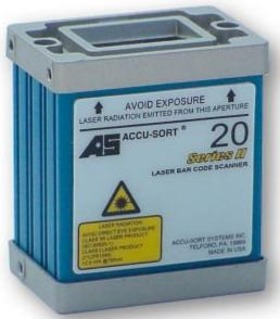
The Model 20II uses an advanced RISC microprocessor to decode scanned data at very high rates and perform various application functions. The standard configuration provides 13 code types with autodiscrimination of eight bar code symbologies at once. Two parallel outputs selectable for valid and non-valid codes provide external signals to operate small relays.
